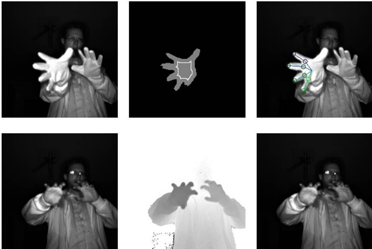
Figure 6: Experimental results. The first row shows the detection capabilities for a hand covered by a glove and an arm covered by sleeves (left: original amplitude data; middle: fine segmentation (gray) and palm contour (white); right: identified fingers, root finger joints and palm center). The second row shows the sensitivity of the processing pipeline: Since the fingers are strongly bent, no fingers are detected as the processing pipeline was designed to detect straight fingers (left: original amplitude image; middle: depth map; right: detection result with no marked fingers).
