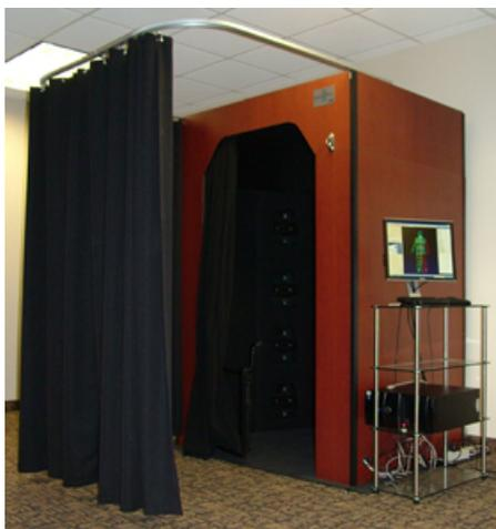
*KX-16 Low Cost 3D Body Scan booth using Kinect Sensors*
