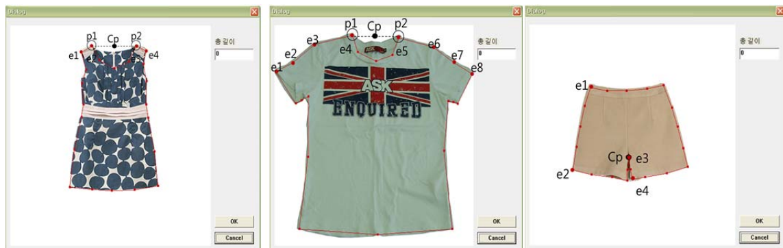
Fig. 1. Extracting front and back images of garment and determining the base point for fitting.
