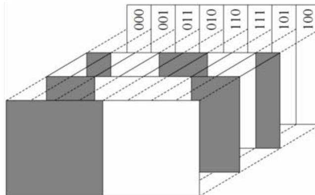
*Fig. 5. Enhanced numeration of stripes through a special encoding of the structured light (Gray code). By projection of a sequence of binary coded stripe patterns, the subsequent light levels for each pixel are forming a unique binary word revealing the individual stripe number. To minimize the effect of bit errors, the stripe patterns are designed to change only one bit per stripe.*
