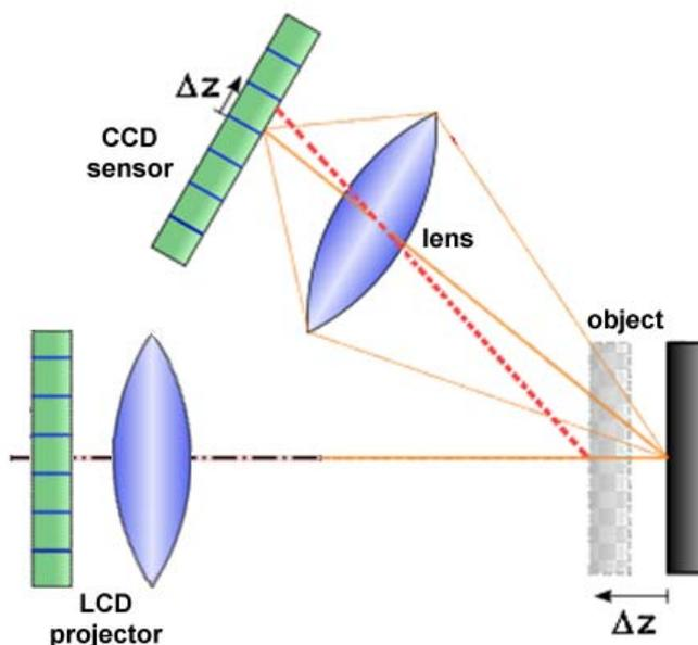
Fig. 3. Principle of triangulation by a couple LCD projector/camera (CCD sensor)
