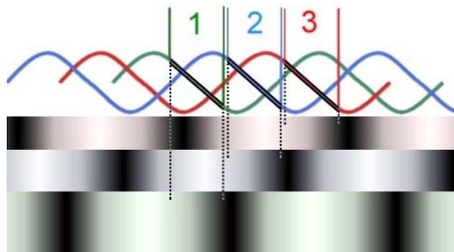
*Fig. 6. Enhanced resolution through the projection of additional patterns (Phase Shifting method)
