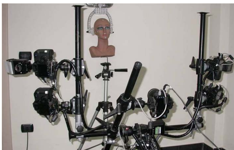
Fig. 1. The FaceshapeMaxi5 3D photogrammetric scanner system developed by Polishape 3D srl
